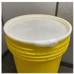
For the drum described above, an HDPE Lid is applied, and then an HDPE Lever Lock ring is applied, closed and sealed with a twist tie or similar device.
